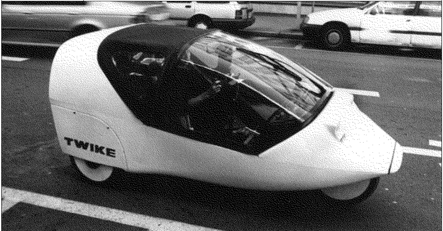
Twike (Twin Bike) A three-wheeled, two-passenger, human/electric-powered ultralight vehicle
